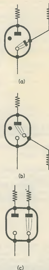
Fig. 2. Methods of priming by means of an auxiliary discharge: (a) with a priming anode, (b) with a priming cathode and (c) with two priming electrodes
